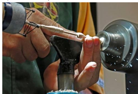
Eli's knitting spool tensioning technique for turning his Tremblers
